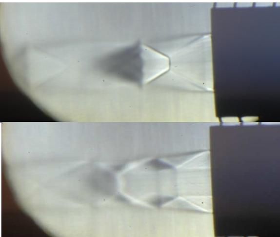
Figure 5: Distribution and Schlieren images at a 6.5 bar inlet.
