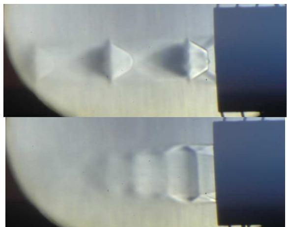
Figure 3: Distribution and Schlieren images at a 4.5 bar inlet
