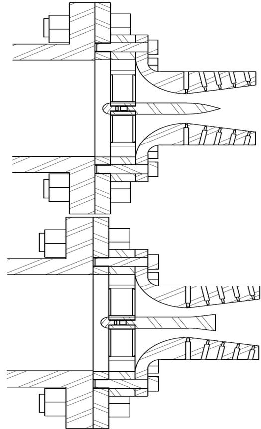
Figure 1: Section views of the converging-diverging and expansion-deflection nozzle configurations.
