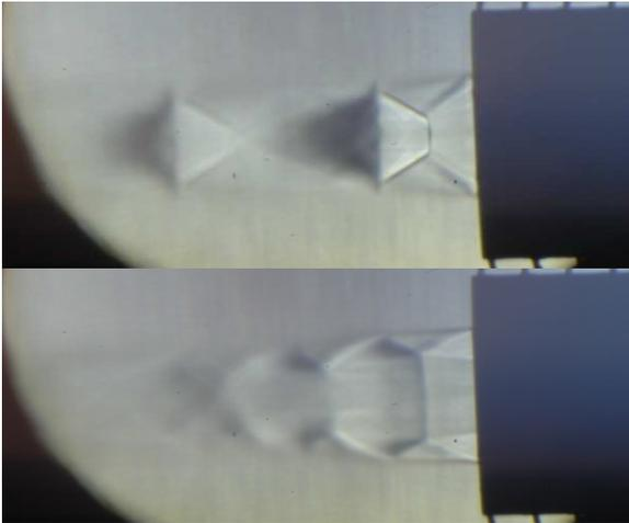
Figure 4: Distribution and Schlieren images at a 5.5 bar inlet
